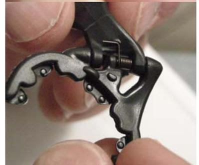
6. Place the hook-end of the safety-pin through the bottom of the cavity and grab the spring leg at the bend (as shown). You can then rotate the harness towards the spring and pull the spring leg through the cavity. Once through, the leg will probably snap into the recess. If not, a slight nudge from your thumb nail will seat the leg. Congratulations! Go jam!
